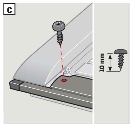
**ENGLISH:** Position bottom cover and push up against bottom edge of profile. Distance **X** must be the same at both sides. Make a mark with bradawl through holes in bottom cover **a**. Drill  $\varnothing 2$  mm holes **b**. Fit bottom cover **c**.
