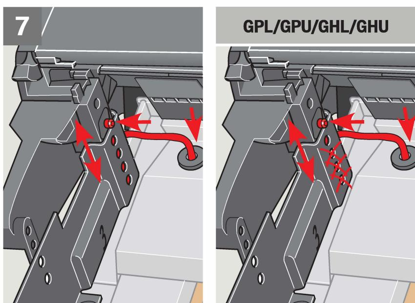
**ENGLISH:** Lower the roller shutter top casing as much as possible. Do **not** press the top casing against the roofing material **a**, **b**. Pull cable through hole on window top cover.
