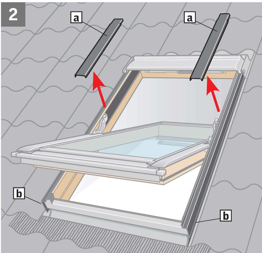
**ENGLISH:** Remove the covers indicated temporarily by releasing the snap locks **a**. Note the position of the covers for later refitting. Do **not** remove side frame covers **b**.
