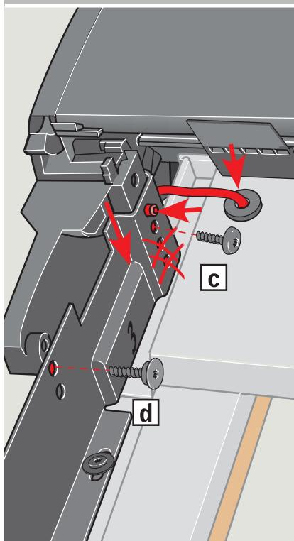
**ENGLISH:** Lower the roller shutter top casing as much as possible. Do **not** press the top casing against the roofing material **a**, **b**. Pull cable through hole on window top cover. Fit securing screws after installing the roller shutter top casing **c**, **d**.
