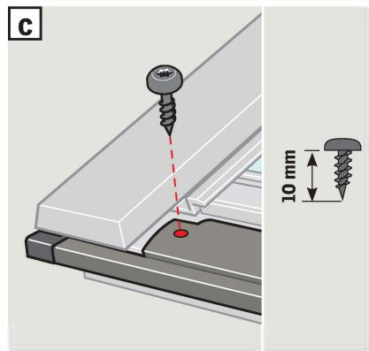
**ENGLISH:** Position bottom cover and push up against bottom edge of profile. Distance **X** must be the same at both sides. Make a mark with bradawl through holes in bottom cover **a**. Drill Ø2 mm holes **b**. Fit bottom cover **c**.
