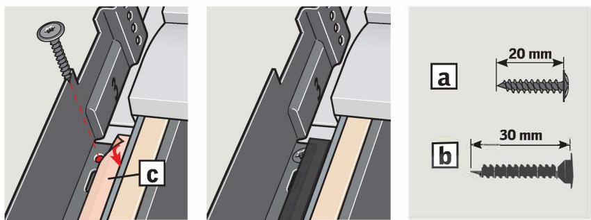
**ENGLISH:** Fix roller shutter side covers in the round holes with screws **a**, **b**.
