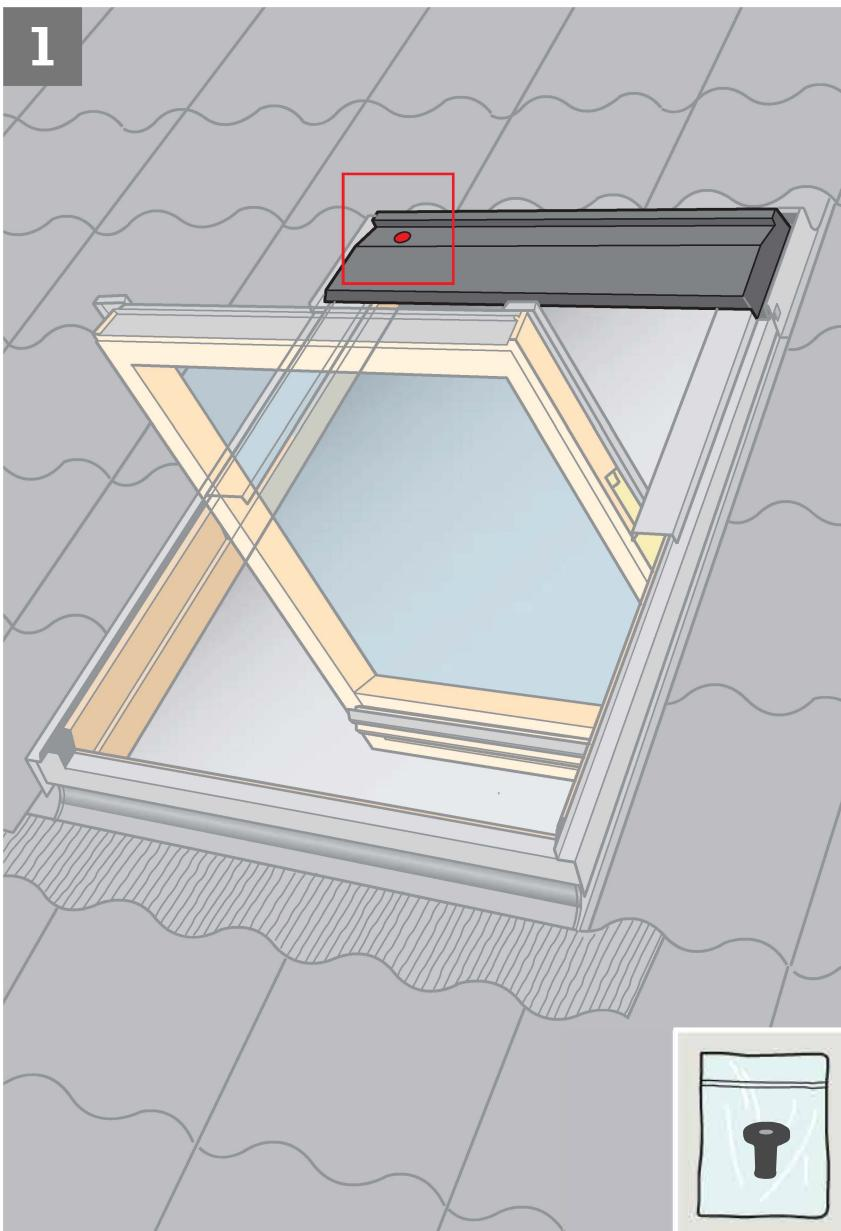
**ENGLISH:** If the window has been fitted with a black screen profile and/or a connection box, remove this/these temporarily **a**, **b**. Drill hole **c** and fit rubber grommet **d**. Pull grommet through from the inside **e**.
