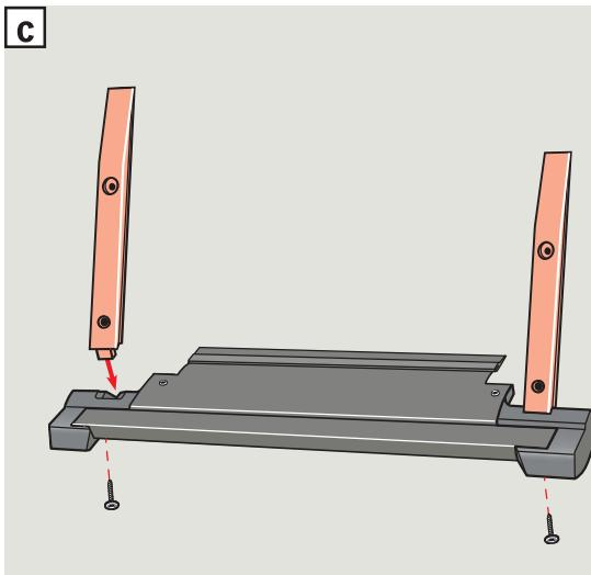
**ENGLISH:** Fit gasket on bottom cover and cut length **a**, **b**. Fit storm brackets to connection pieces **c**.
