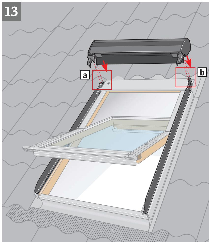
**ENGLISH:** Fit roller shutter top casing into grooves on side covers **a**. Check that rubber gasket at the back fits smoothly against outside of window **b**.
