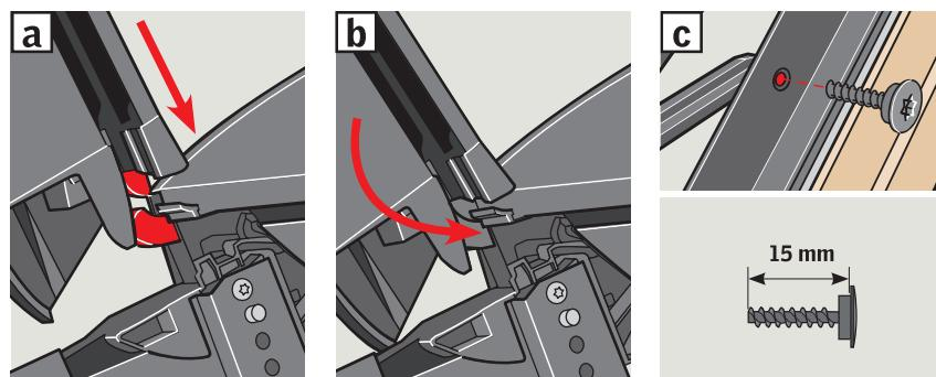
**ENGLISH:** Fit plastic insert pieces on the roller shutter side channels **a**, **b**.
