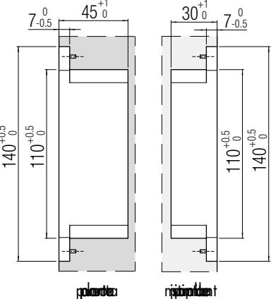
**Installation of hinge (without door leaf)**
