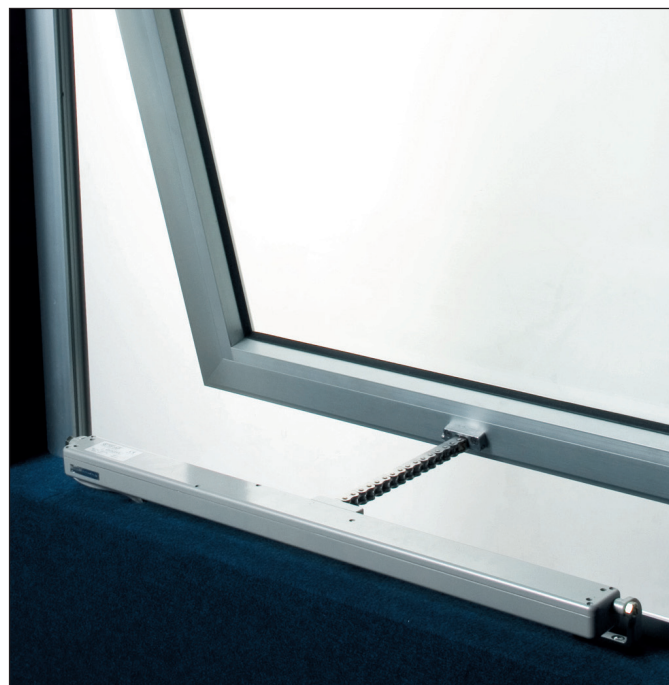
SYNCHRO QUASAR DC DRAWBRIDGE Installation on bottom hinged window, opening outwards 90°. The actuators are equipped with a special guide for the chain. Contact our Technical Department for the installation limits (size and weight of window) and brackets for actuator installation (depending on type of profile)
