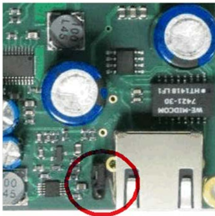
Power supply via PoE The jumper is on the two top pins.
